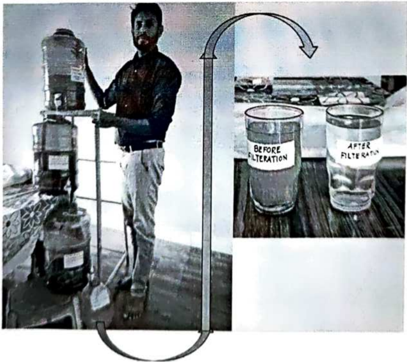
Figure No. 8: Greywater Treatment System with a sample before filtration and after filtration
